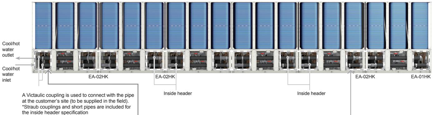
A Victaulic coupling is used to connect with the pipe at the customer's site (to be supplied in the field).
