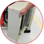
Hinged speed drivers boxes for an easier access to each internal component
