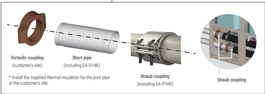
\* Install the supplied thermal insulation for the joint pipe at the customer's site.
